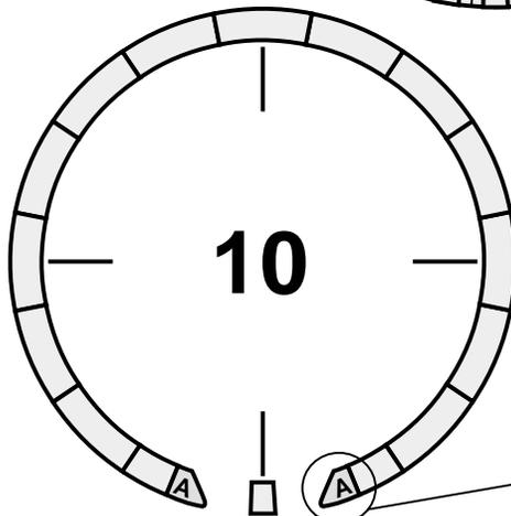
Broken arrow slit blocks on each side
